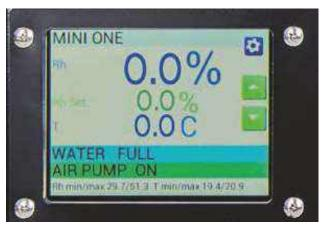
Ambient gallery air is filtered for pollutants and drawn into the unit. This air is pressurized and directed through a proprietary mechanism that adjusts the relative humidity to the pre-set valueThis air is directed through a small flexible tube to an input port in the showcase. Air flow to the enclosure is constant, and in normal applications the air is delivered only at the preset relative humidity.
