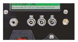
The Minione is equipped with two external alarms: one for "Out of Range [RH]" and one for "Low water [LW]" status.
